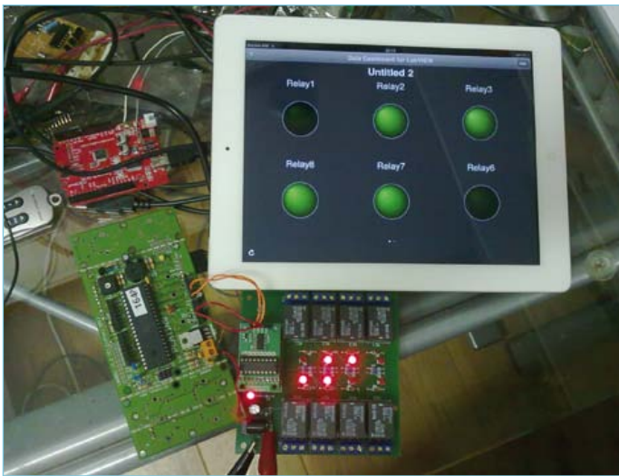
Figure 4. This is the 8-channel relay board with synchronous serial interface that I want to control from LabVIEW.
