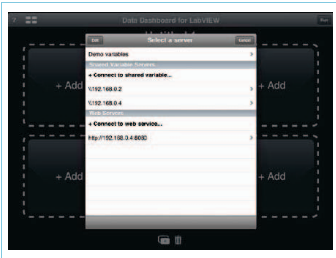
Figure 10. The server selection window in Data Dashboard on an iPad. If your server is listed, tap it, if not tap Connect to shared variable.
