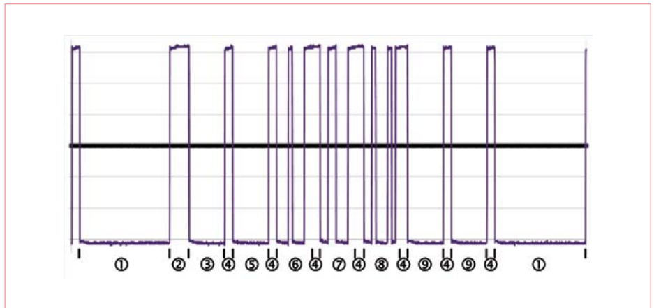
Figure 5. This DMX timing diagram shows a data block composed of the following parts:
