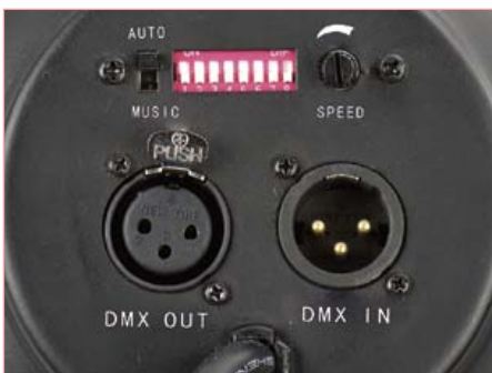
Figure 6. The input and output DMX connectors on the rear of the RGB LED spotlight. The DIP switches are used to set the DMX communication channel for the lamp.
