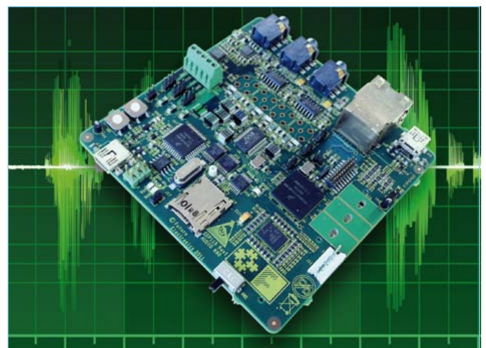
Photo 1. The audio streaming board by Future Electronics is based on a Freescale Kinetis K60 with ARM Cortex-M4 core.
