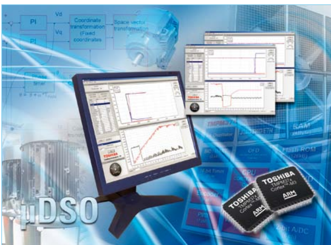
Photo 2. Toshiba has integrated a digital storage oscilloscope ( \mu\text{DSO} ) in its Cortex-M3 based MCU for motor control applications. Is this the start of a new trend?
