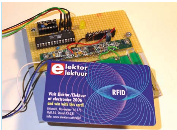
Figure 4. Prototype with ATmega88 and PN512 reader board.
