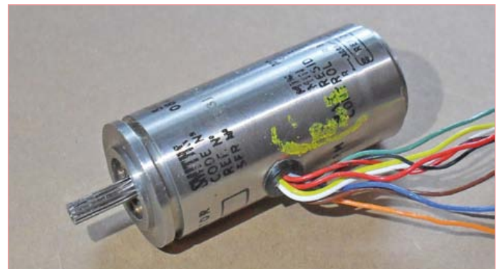
Figure 8. One of the motor/tachogenerators units.
