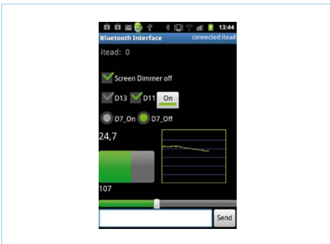
Figure 6. The interface in use. The messages sent by lthead (the Bluetooth shield) or Me (the phone) are visible at the top. Commands to be sent can be entered manually at the bottom. These features are handy for troubleshooting, but you may want to remove them for other applications.
