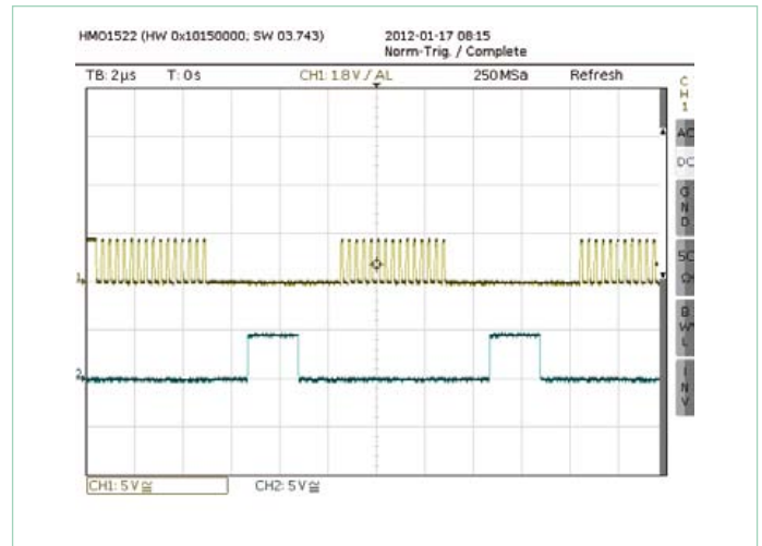
Figure 6. Measuring the execution time of the interrupt service routine.
