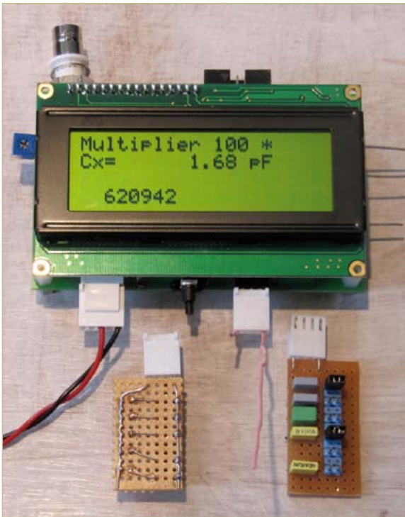
Figure 3. It is any good? The author's prototype gets 'grilled' for accuracy using an array of capacitors and test fixtures. Note the use of a 4x20 LCD, which turned out very useful for diagnostic purposes.
