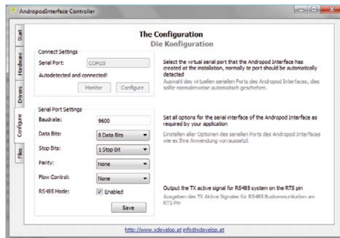
Figure 9. Serial interface configuration for connecting your own circuitry.
