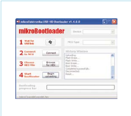
Figure 3. If there is a bootloader present in the microcontroller, the mikroBootloader makes it possible to load a new executable in record time.
