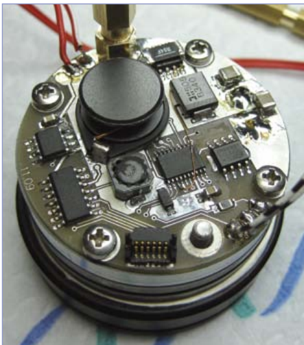
Figure 3. The circular double sided PCB takes SMD components.
