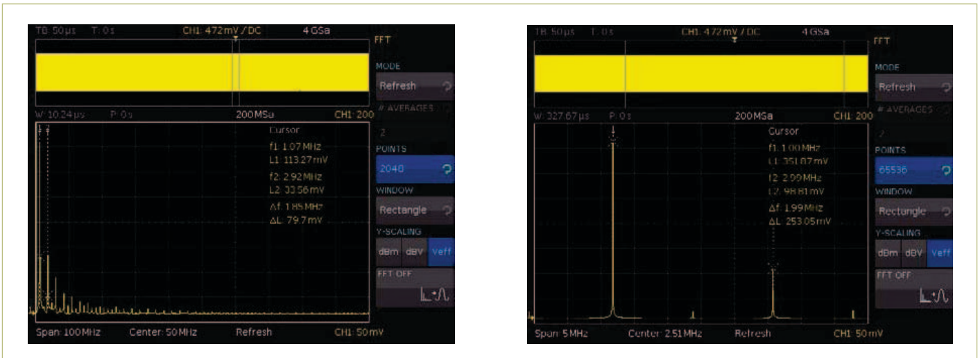
Figure 3. An FFT feature is only really practical if it uses a sufficient number of points for the calculations (left 2048 Points, right 65536 Points).
