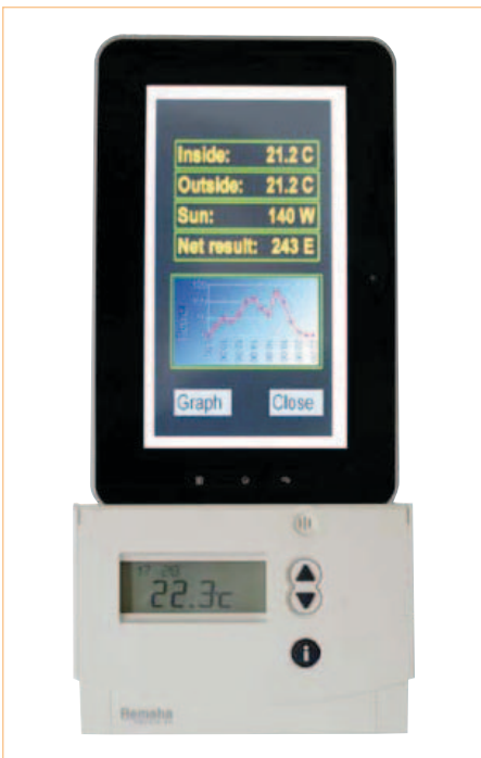
Figure 3. Using a tablet in a home automation system.
