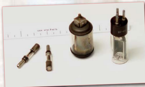
“Miniature” phototubes were one of the innovations that made sound movies possible in the 30s. Optical sound tracks recorded the audio information on the edge of the film. Later sound systems used magnetic stripes, which resulted in improved sound quality.
