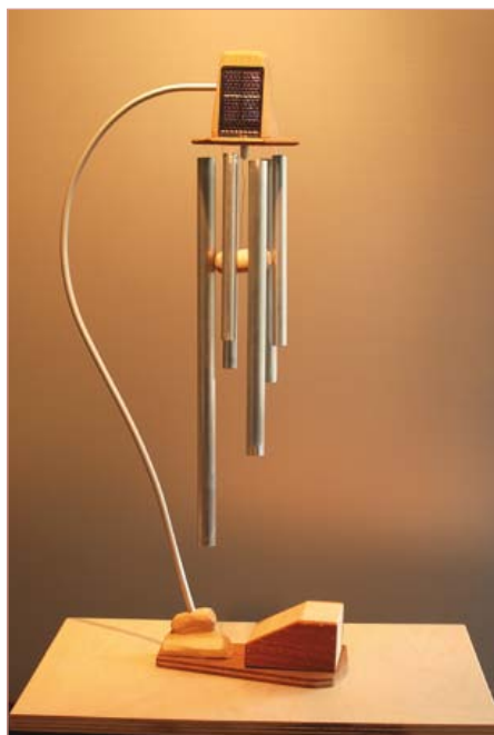
Figure 3. The chime sounds when enough energy has been harvested. This saves watching the meter all the time.
