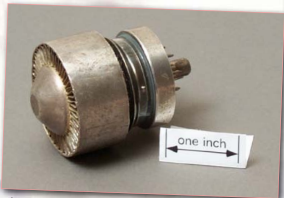
A 4X150 tetrode power transmitter tube. The metal anode has integral fins for forced-air cooling. Very famous — “every radio amateur has one”.
