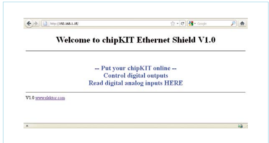
Figure 4. The result of a successful port: I can now connect to a tiny web server running on the Max32.
