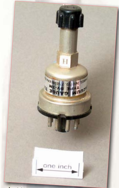
Inside this tube is a heater and a thermocouple, which generates a tiny vacuum-dependent voltage. An 1/8" NPT fitting connects to the vacuum system.
