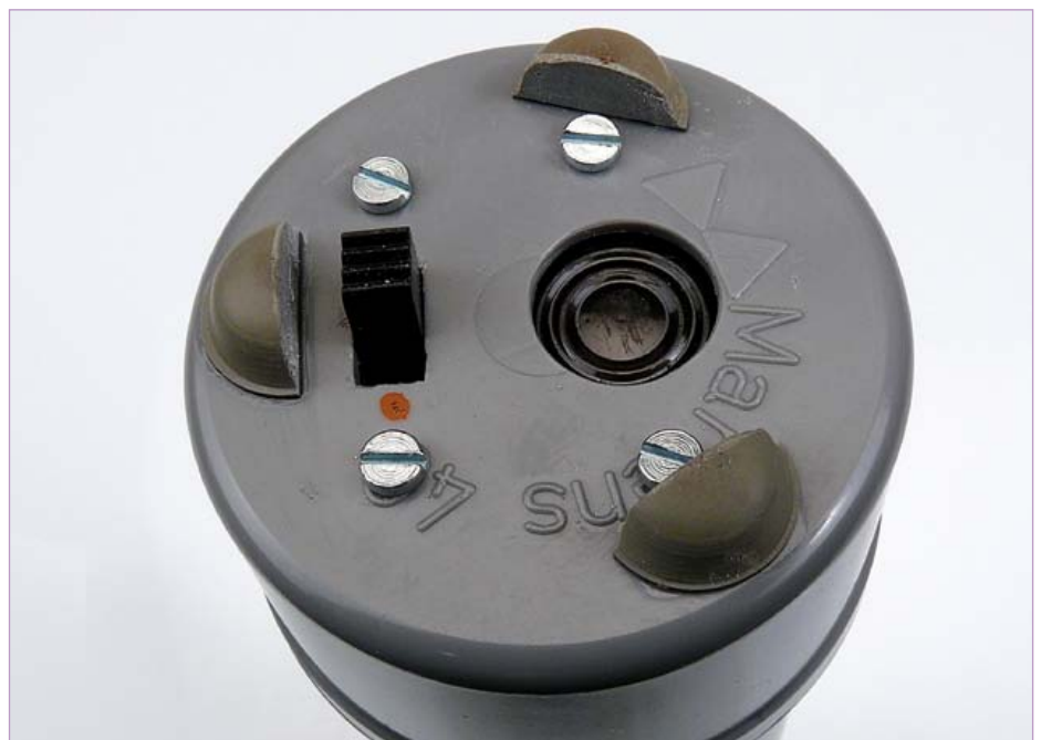
Figure 4. The on/off switch and a speaker are fitted in the end cap.
