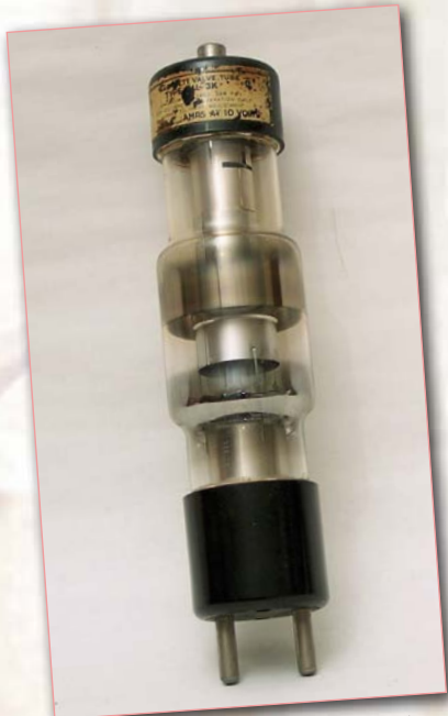
This 1950s X-Ray tube is about a foot long. It has a fixed anode and cathode. Modern tubes increase power by using a large anode that rotates at a high speed.
