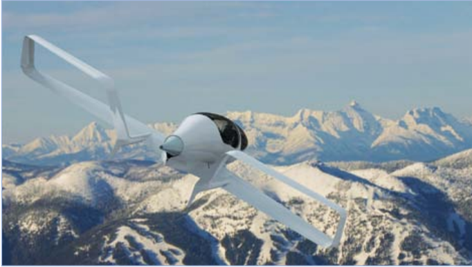
Figure 5. The 6-seater Synergy will take part in the GFC powered by its 142 kW (193 HP) bio-diesel motor. Image: CAFE Foundation Blog.
