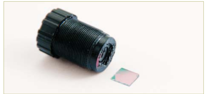
Figure 3. With the König lens the removal of the IR filter was quite easy to do.
