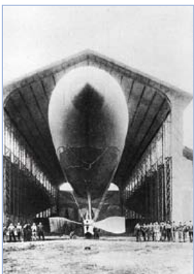
Figure 1. Pure innovation: The airship 'La France' in 1884, it was the first steerable airship, the first to have electric drive and the first to use Redox flow Batteries. Image: Wikimedia Commons/Photo (1885), 2001 National Air and Space Museum, Smithsonian Institution.
