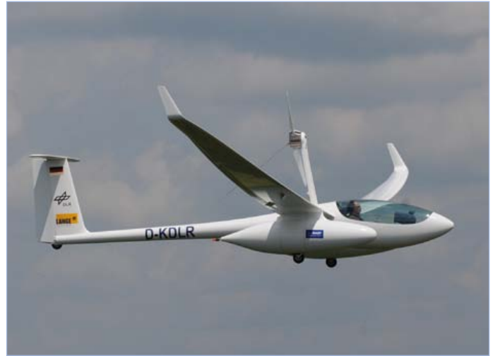
Figure 2. The Antares 20E from Lange Aviation — shown is the DLR-Version with hydrogen tank and fuel cell in pods slung beneath the wing. Image: DLR.
