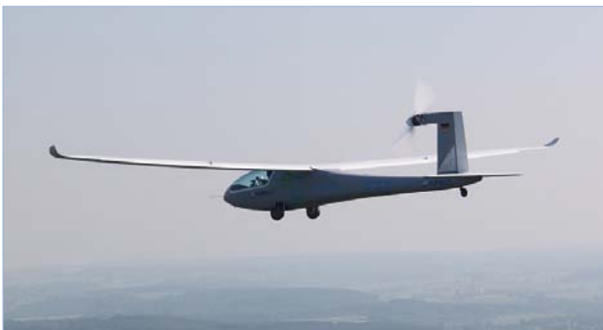
Figure 8. Originally the ‘Hydrogenius’ this fuel cell concept e-Genius from Stuttgart University is a very efficient electric flyer competing in the GFC contest. Image: e-Genius-Team, IFB University Stuttgart.
