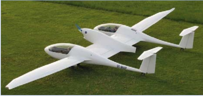
Figure 7. Pipistrel from Slovenia has combined two Taurus motorgliders together with a 145 kW electric motor to make this twin-fuselage entry for the GFC. Taking advantage of the ‘per passenger’ calculation of fuel allowance. Image: Pipistrel.
