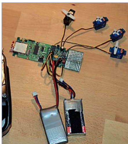
Figure 5. Author’s prototype connected to four servos and two LiPo batteries.
