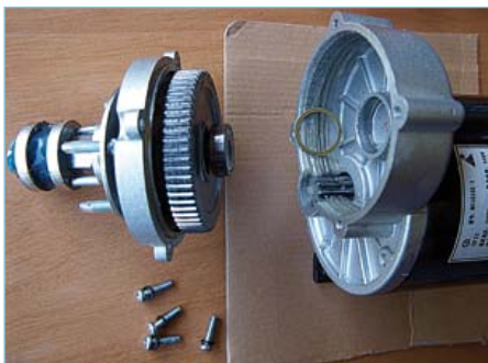
Figure 8. Release the four bolts and carefully remove the casing which holds the stub axle and the final drive gear wheel.
