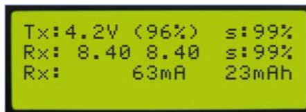
Figure 4. This is what the display shows when powering the transmitter from 4.2 V and the receiver from two 8.4 V batteries.
