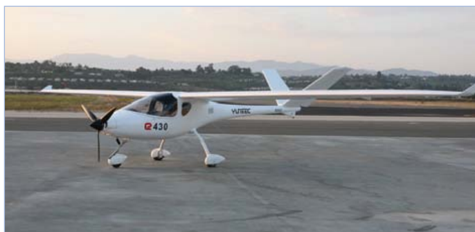
Figure 3. The Yuneec E430 is the first electric aircraft from China developed by a model aircraft manufacturer. Image: Yuneec.
