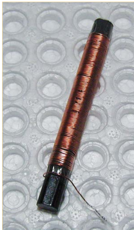
Figure 5. A radio ferrite rod makes a good core for winding a 60-160 \mu\text{H} adjustable inductor that enables the largely capacitive transducers to be peaked at their resonant frequency (usually, 40 kHz).
