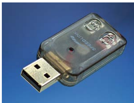
Figure 2. The converter is formed from a modified and recycled 'Ultra Portable Audio Card' from Speed-Link.
