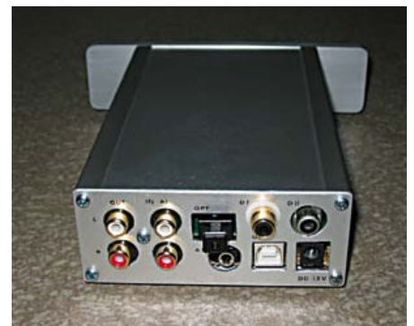
Figure 1. The converter offers a very simple method of fitting a USB input to an external D/A converter. (The author's audio equipment is shown here, see [1])
