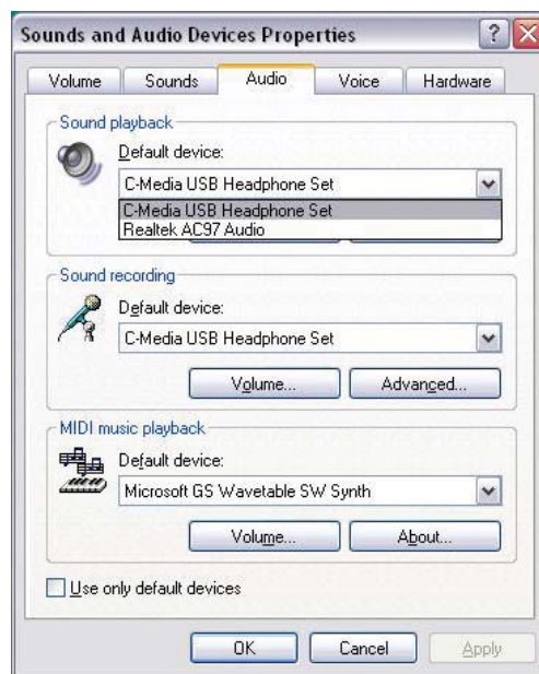
Figure 4. The adapter is recognized as a soundcard chip once it is plugged into a USB port on the PC. Audio can be routed through the internal sound card, through the adapter or through any additional audio equipment.
