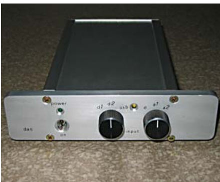
Figure 1. The converter offers a very simple method of fitting a USB input to an external D/A converter. (The author's audio equipment is shown here, see [1])
