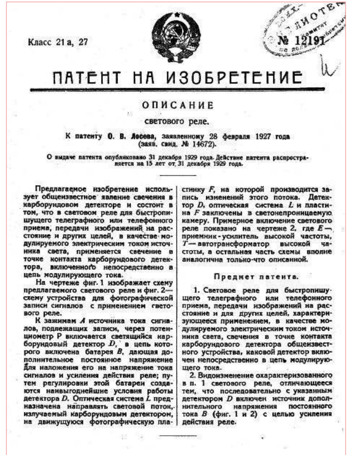
Figure 4. USSR patent issued to Oleg Losev in 1927 for his 'light relay' system (courtesy PatentsFromRU.com).
