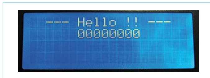
Figure 7. Hello, all the relays are de-energized.
