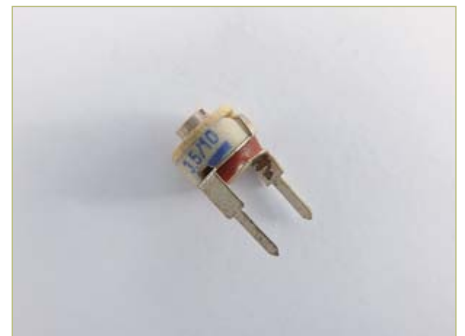
(f) Ceramic trimmer capacitor. 3.5–10 pF adjustable.
