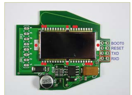
Figure 10. The pins to be soldered are marked here. None of the other pins is needed.
