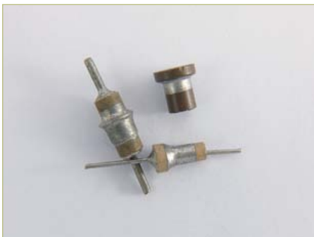
(d) Feedthrough capacitors. Low stray inductance. Ideal for RF decoupling. 200 pF, 470 pF, 1 nF.
