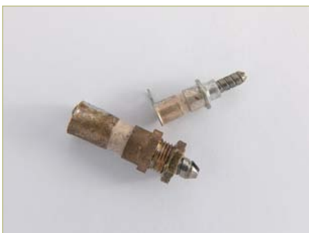
(g) Tubular trimmer capacitors. Unless in series, the rotor is best grounded. 0.3–3 pF, 1–6.5 pF.
