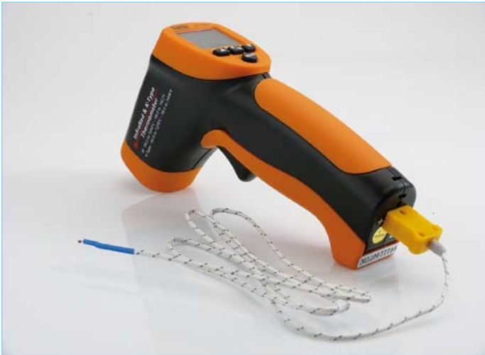
Figure 6. Some instruments come with a type K thermocouple, which can be used as contact sensor to measure the surface temperature so that the emissivity setting can be adjusted for IR measurements.
