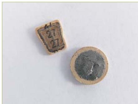
(e) Coffin and disc capacitors. Low loss factor, zero stray inductance. On-PCB coupling and decoupling. Fragile devices! Connect straight to a PCB track and copper earth plane. 27 pF, 820 pF.
