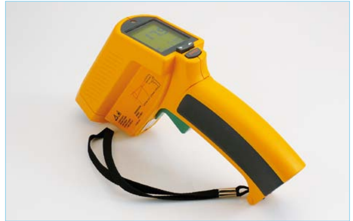
Figure 4. We used this Fluke 572 IR thermometer as a reference for our tests. It has a 50:1 FOV.
