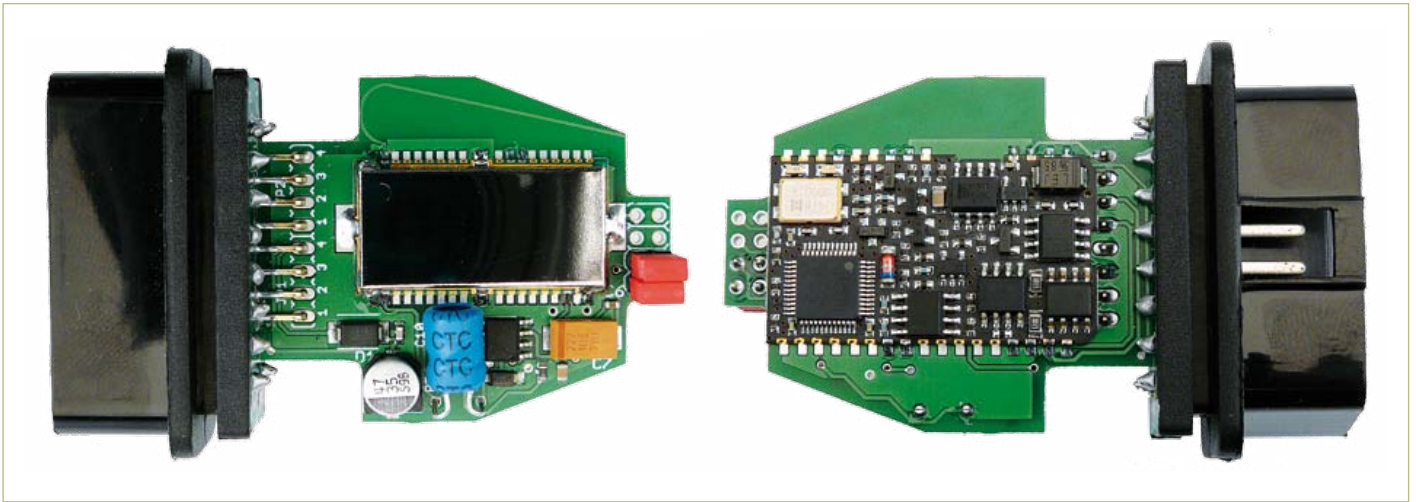
Figure 3. Top and bottom sides of the Bluetooth interface board with OBD plug soldered on.
