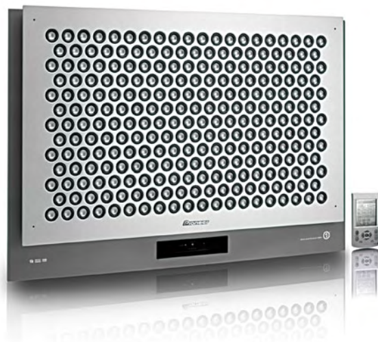
Figure 5. The Pioneer PDSP-1 digital sound projector sports 254 transducers (and 254 digital amplifiers), but unfortunately is no longer available.
