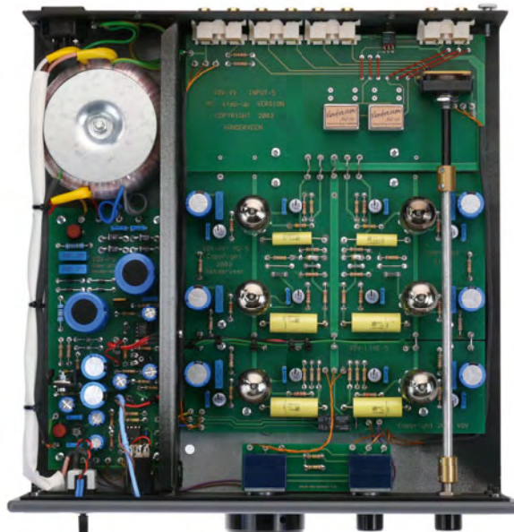
Figure 1. Interior view of the MCML05 preamplifier. The special MC transformers can be seen at the rear, next to the input connectors.
