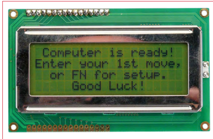
Figure 5. When power is applied the computer invites you to enter your first move.
