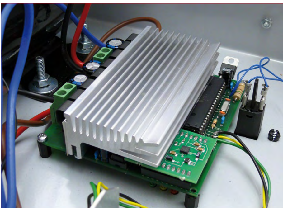
Figure 5. The compact electronics module comprises the main board with heatsink and sensor daughter board.
