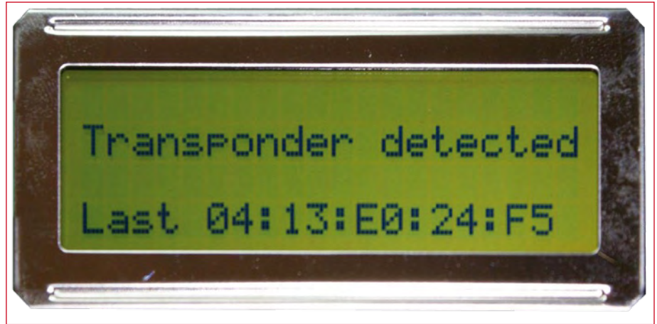
Figure 11. When a RFID tag is recognized, the data read from the tag is shown on the LC display.
