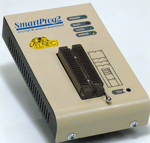
Figure 1. Elnec's SmartProg2 was used for a number of years in the Elektor Labs for one-off microcontroller programming and small production batches.
