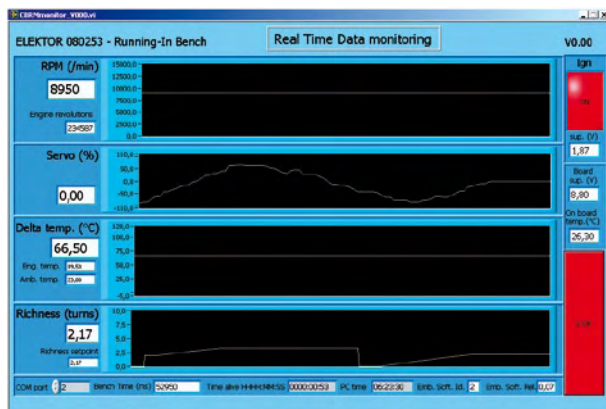
Figure 9. The CBRMmonitor software for PC shows the key engine parameters live as they change.
