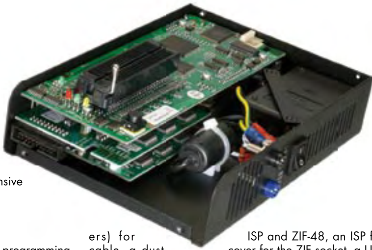
Figure 3. A look inside the BeeProg+ – a very powerful microcontroller system on its own!
