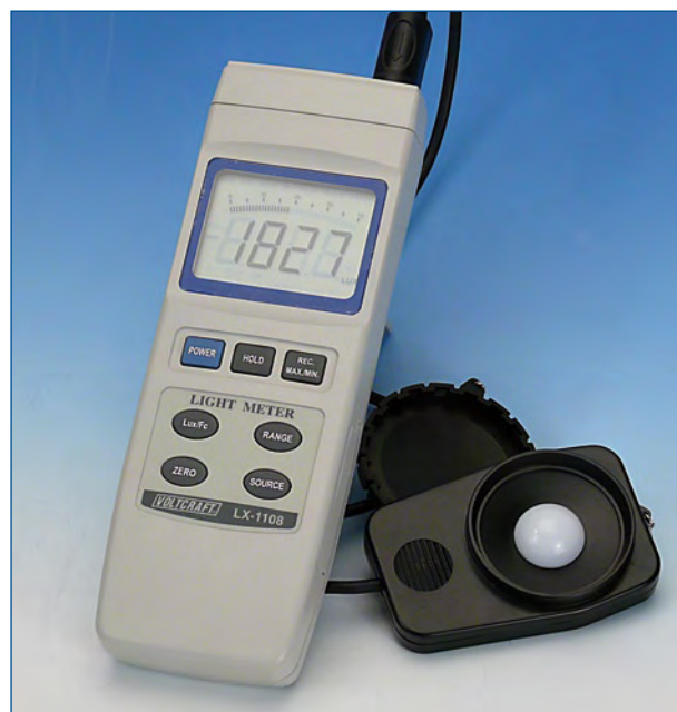
Figure 2. A light meter calibrated in lux is indispensable for measuring light intensity. For our measurements, we used a Volcraft LX-1108 provided by Conrad Netherlands.
