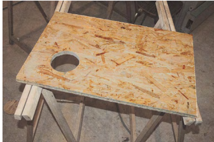
Figure 11. A solid panel of wood lets you fix the bench onto trestles.
