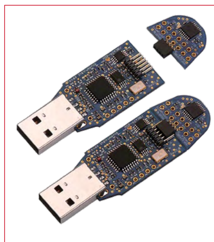
Figure 1. The eZ430 evaluation stick, around which this experimenter's system is based.
