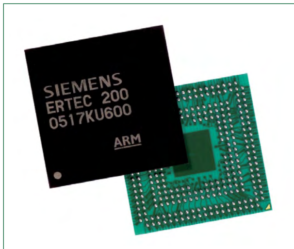
Figure 3. A Siemens ERTEC 200 processor with a built-in ARM processor and two Ethernet interfaces. Source: Siemens
