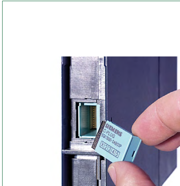
Figure 1. A Siemens C-Plug with a capacity of 32 MB. Source: Siemens
