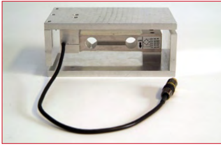
Figure 6. This commercial bending beam strain gage measures both horizontal and vertical force.
