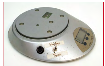
Figure 5. The switch allows the scales to revert back to normal weighing duties.
