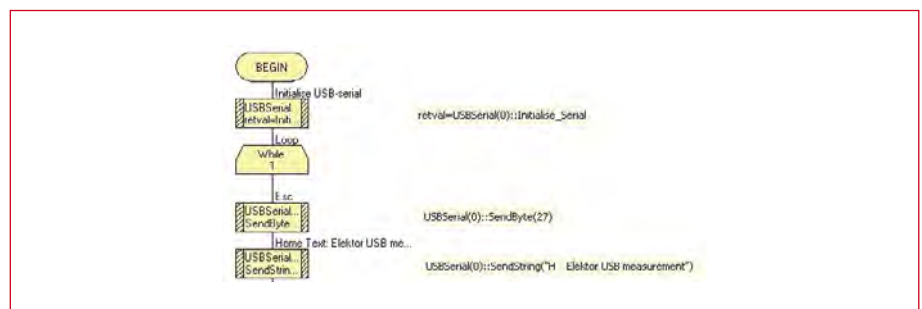
Figure 4. Flowcode for the initialisation of the USB connection and displaying the first line of text.
