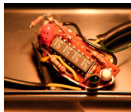
Figure 10. The PC817 quad optocoupler is by far the largest part in the PC interface.
