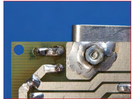
Figure 6. For lower power applications it is sufficient to solder an M3 nut to the pad on the reverse of the printed circuit board to help dissipate heat.
