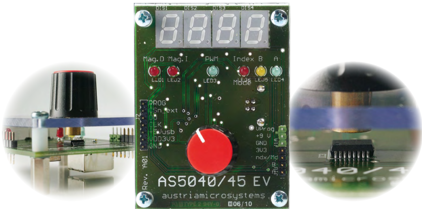
Figure 6. An AS50xx demonstration board provides a development environment for dedicated applications using its accompanying free software.
