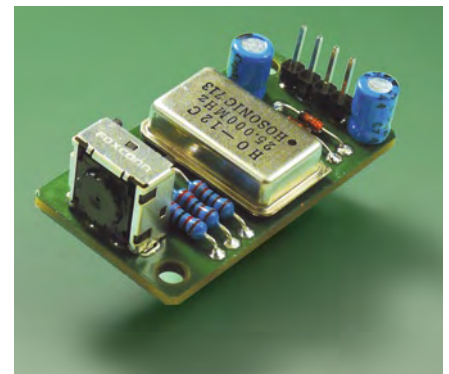
Figure 10. Lab prototype of the PCB with the camera sensor.
