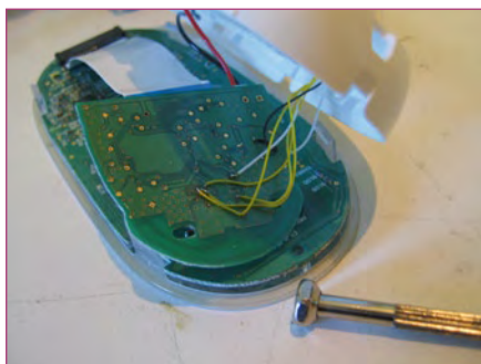
In the remote control we find two printed circuit boards that are interconnected with a ribbon cable.
