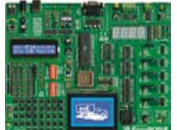
Easy8051B Development Board with on-board USB 2.0 programmer
