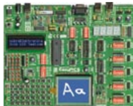
EasyPIC5 Development Board Complete Hardware and Software solution with on-board USB 2.0 programmer and mikroICD
