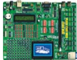
Uni-DS 3 Development Board Complete Hardware and Software solution with on-board USB 2.0 programmer
