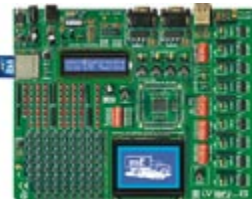
LV 18FJ Development Board Complete Hardware and Software solution with on-board USB 2.0 programmer and mikroICD
