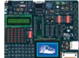
EasyPSoc3 Development Board with on-board USB 2.0 programmer
