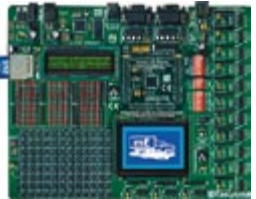
EasyARM Development Board Complete Hardware and Software solution with on-board USB 2.0 programmer
