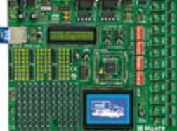
BIGAVR Development Board with on-board USB 2.0 programmer
