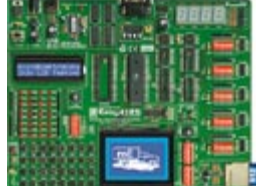
EasyAVR5 Development Board with on-board USB 2.0 programmer
