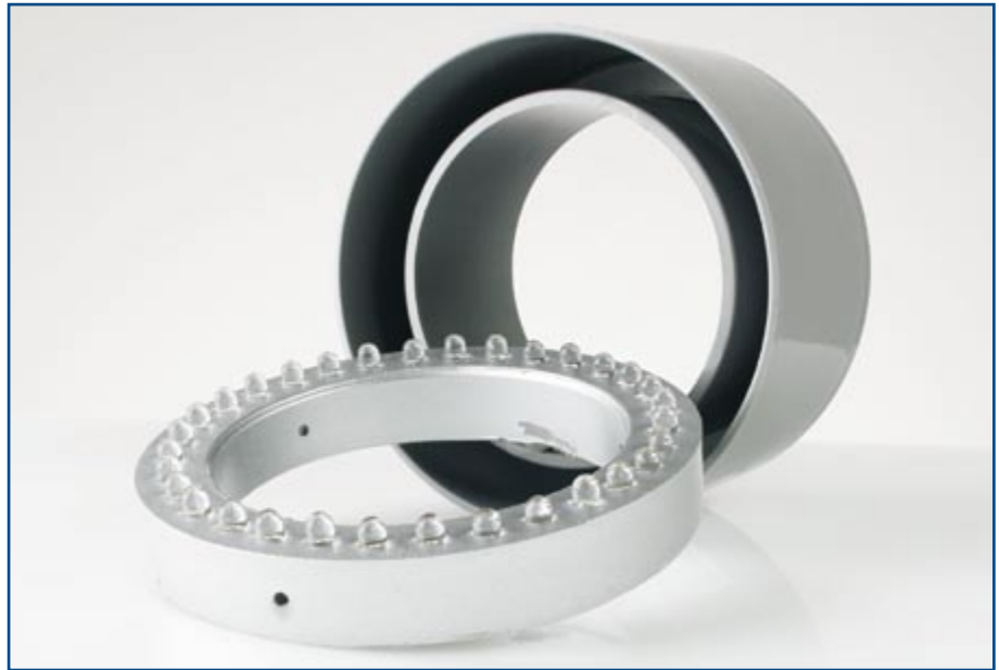
Figure 5. Our LED ring started life as a pipe connector found in many DIY stores.
