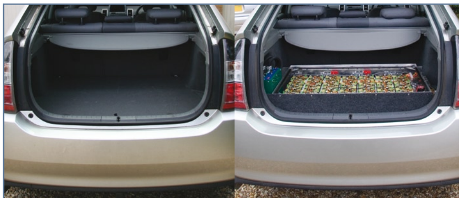
Figure 5. 'Before' (left) and 'after' (right) pictures of the battery system.
