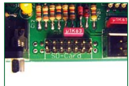
Figure 5. In order to fit an SD memory card between the pins of the DIL header connector the pins of each row are bent inwards until they stand about 1.5 mm apart.
