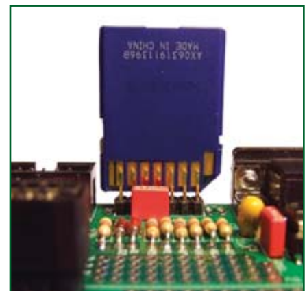
Figure 6. An SD card fitted between the pins of the DIL header connector.
