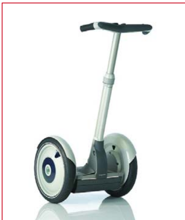
Figure 1. Devices such as the Segway depend on gyroscopes to balance themselves.
