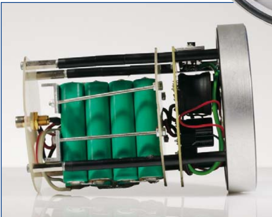
Figure 4. A number of spacers and long screws give a solid construction and a snug fit in the housing
