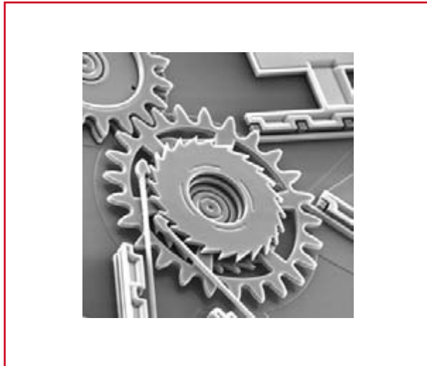
Figure 7. With a little work it is possible to construct working drives using MEMS technology.
