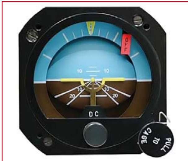
Figure 3. The artificial horizon in an aircraft cockpit contains a gyroscope mounted on gimbals. The gyroscope wheel is electrically or pneumatically driven.
