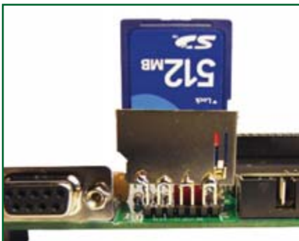
Figure 9. Improved mechanical stability is the result of soldering the electrically 'dead' pins of the header connector to the metal shielding of the SD card slot.
