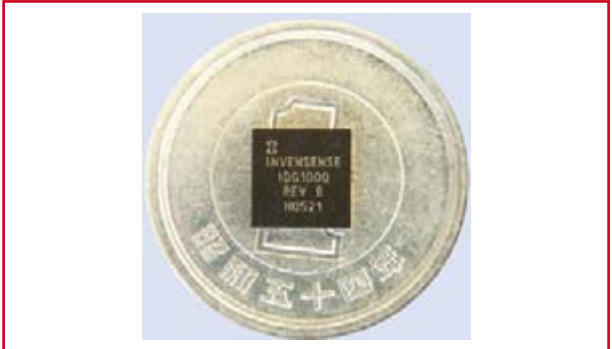
Figure 10. The IDG1000 two-axis gyroscope measures 6 mm by 6 mm.
