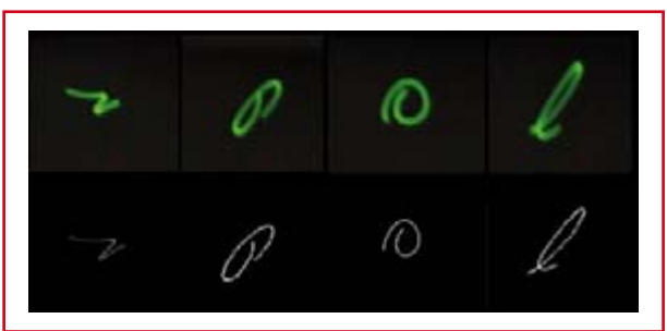
Figure 12. Camera shake, actual and as measured with a gyroscope.
