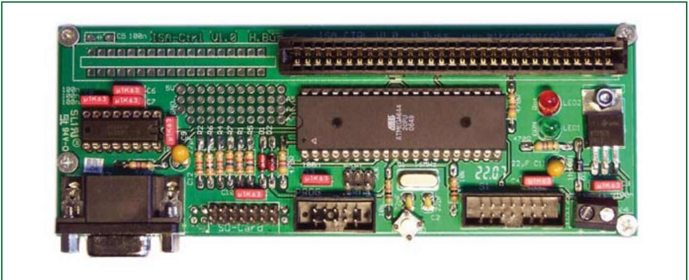
Figure 4. The fully populated web server, with room between the two ICs for future expansion developments.
