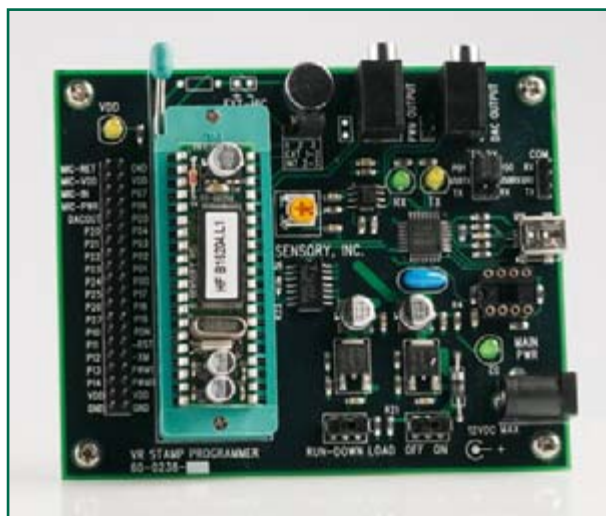
Figure 1. The VR Stamp™ Toolkit is in fact a mother board, onto which the VR Stamp™ Module is piggy-backed.
