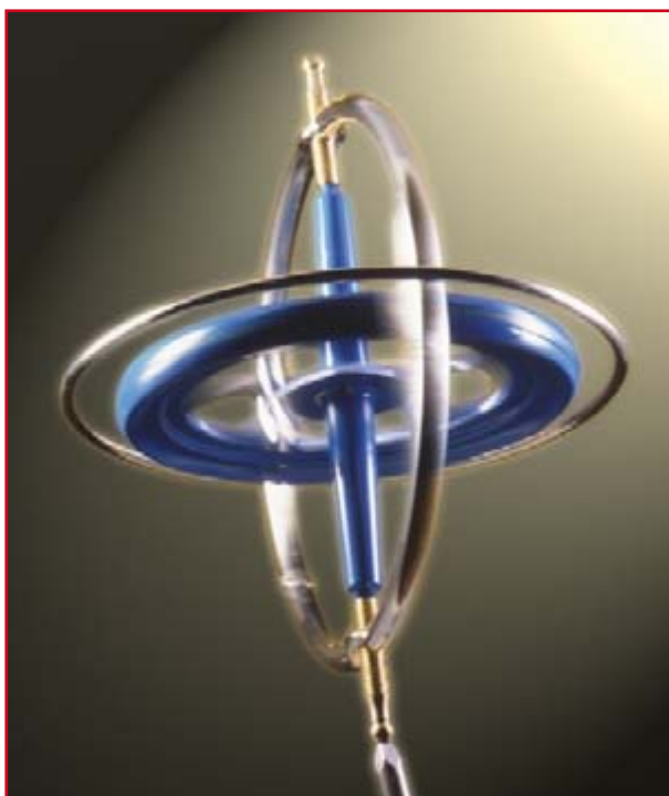
Figure 2. Thanks to the Coriolis force a spinning gyroscope can easily be balanced on the point of a needle.
