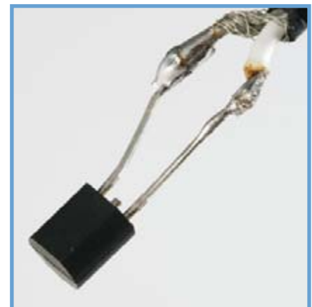
Figure 4. Shielded cable is used for the KTY81 sensors.
