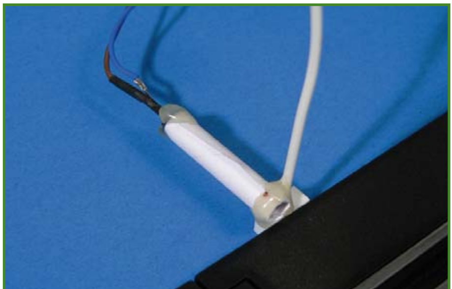
Figure 4. One of the mounted phototransistors (at least one lead of which needs to be insulated) in position, held with a few spots of hot-melt glue.
