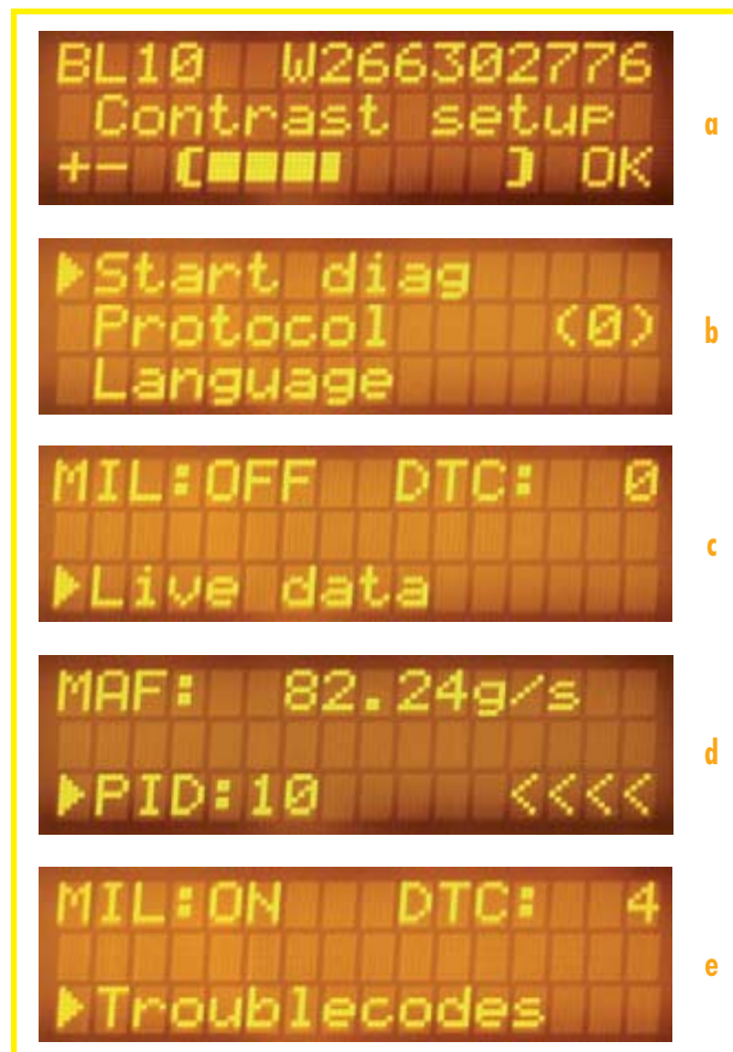
Figure 9. Displays: (a) Contrast setting, (b) Start menu, (c) Status display, (d) MIL/DTC PID Menu, (e) DTC trouble code number.
