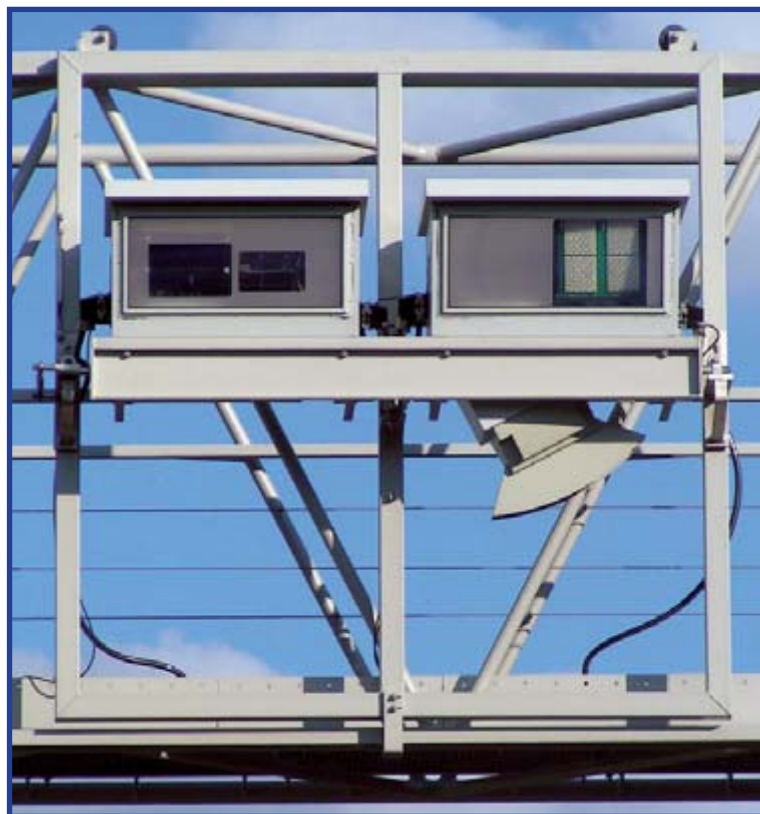
Figure 3. Big Brother's little helpers: cameras on gantries over German autobahns being introduced to log vehicle movements. Similar systems are being trialled in the UK. photo: Stefan Kühn ( www.webkuehn.de ).
