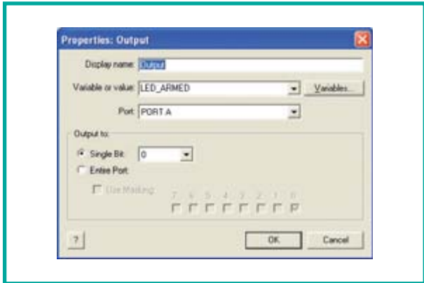
Figure 6. Output 0 of port A goes high to indicate the change of status.
