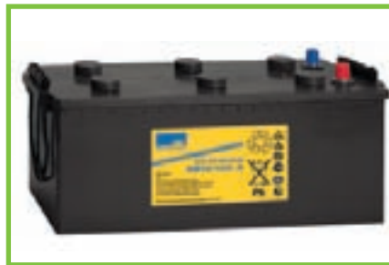
Figure 3. 'Solar batteries', unlike conventional lead-acid batteries, are genuinely maintenance-free and are less prone to self-discharge (photo: Deutsche Exide GmbH).
