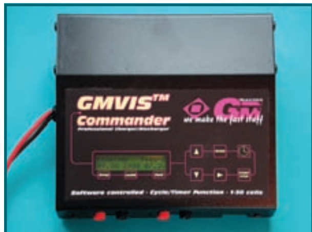
Figure 7. This charger, made by Graupner, allows constant current/constant voltage charging with a current limit at 9.2 A and a maximum charge voltage of 3.6 V per cell.
