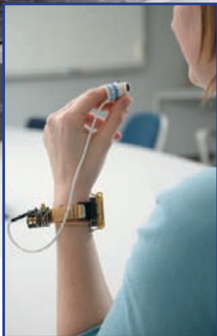
Figure 1. The prototype of the pulse oximeter is already small enough to be worn as a wristwatch.
