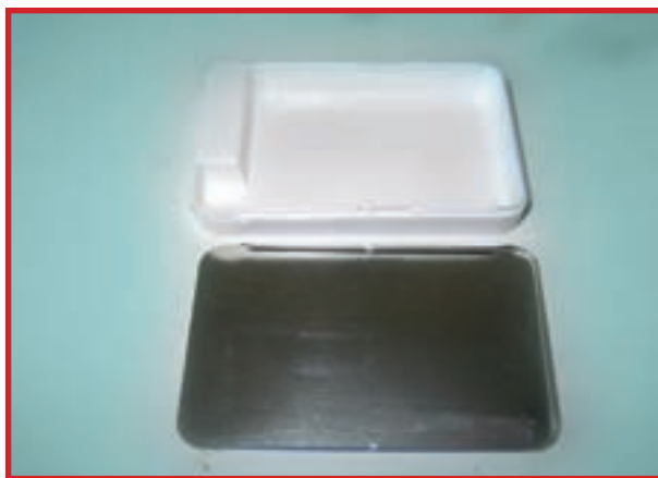
An empty breath refreshers tin was used for the enclosure. It's just big enough to take three AAA batteries, the circuit board and the connector.
