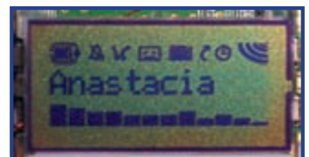
Figure 8. Display of artist name and spectrum analyser output from Winamp on the Alcatel LCD.
