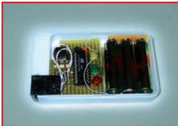
It fits exactly. The black cube on the left is the UTP connector.
