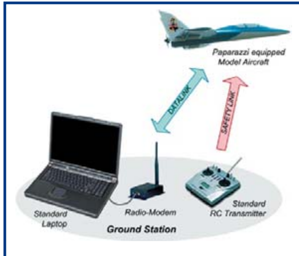
Figure 1. The 'Open-source UAV' ground station consists of a laptop with a radio modem for communication and a standard R/C transmitter for autopilot backup.
