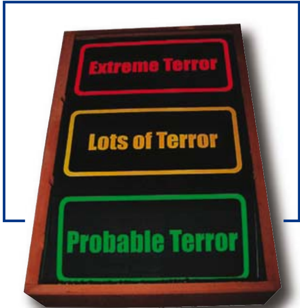
The lighting is provided by a number of bright LEDs, which have been fixed to the case using a hot glue gun. It is of course also possible to use a CCFL or even a 12V incandescent lamp.
