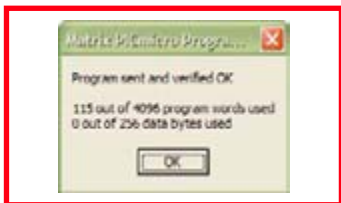
Figure 7. Programming takes only a few seconds. The chip memory still has plenty of space left. As soon as this message pops up, your program starts running.
