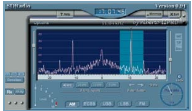
Figure 7. Image frequency with only one mixer.
