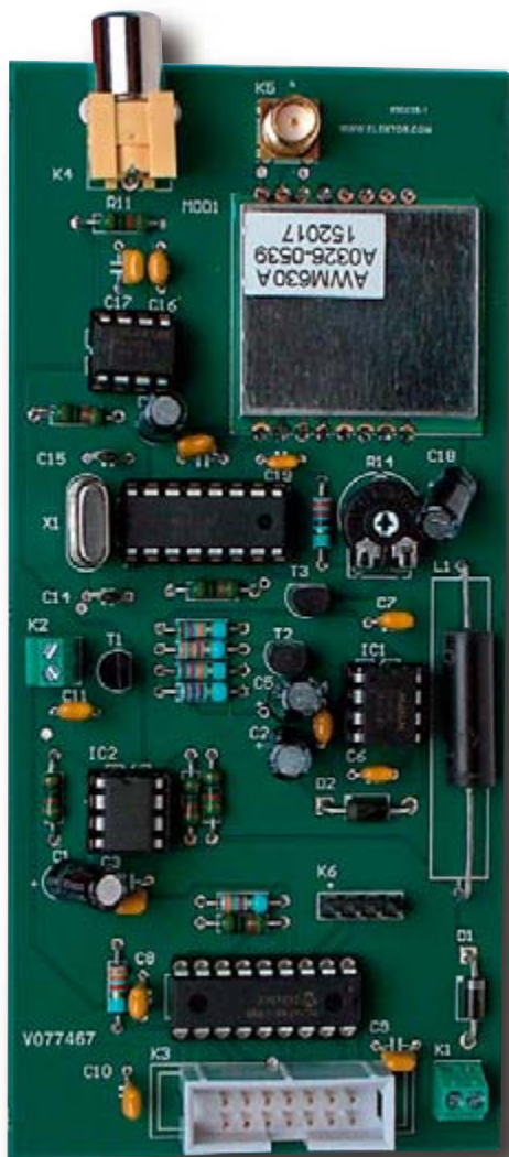
Figure 5. Components mounted on two of our prototype boards. Above: transmitter; below: receiver.
