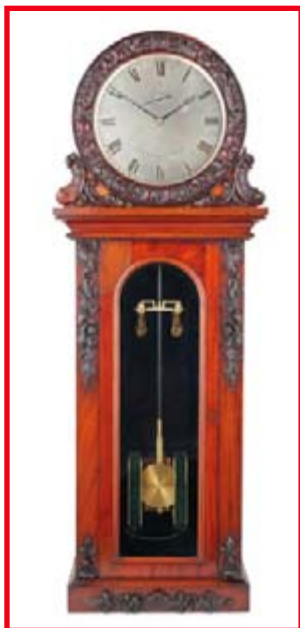
Figure 3. The first electrical clocks used pendulums in conjunction with electromagnets. This example, by Alexander Bain, was made in 1845. Since there was no mains electricity at that time, the maker constructed his own 'earth battery' by burying two sheets of dissimilar metals in the ground. (Photograph: German Clock Museum, Furtwangen [14])
