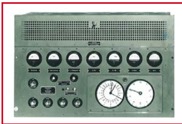
Figure 4. In 1938 Rohde and Schwarz brought their 'portable' quartz crystal clock to market. It weighed some 60 kg! (Photograph: Rohde and Schwarz [4])
