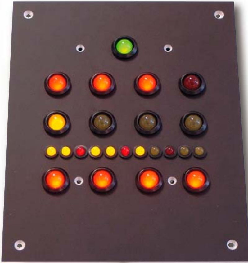
Figure 2. The display of our version uses LEDs instead of lamps.
