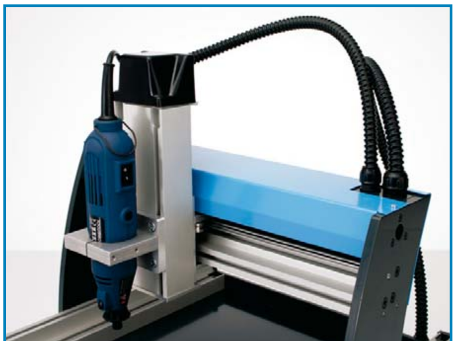
Figure 5. The boring column and the guideway in the bridge.
