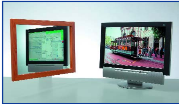
Figure 4. Viewing a television programme and the Internet at the same time on a single LCD: this special Sharp display could solve space problems. (Photo: Sharp)
