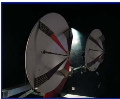
Figure 5. An impulse radiating antenna developed by TNO, Netherlands.
