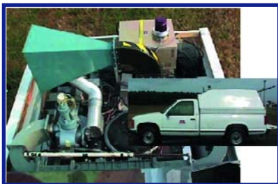
Figure 2. An HPM system fitted in a vehicle.
