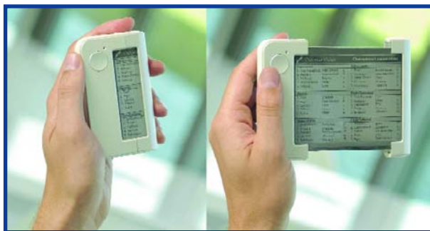
Figure 6. Philips exhibited an OLED-based flexible display at this year's IFA. (Photo: Philips)
