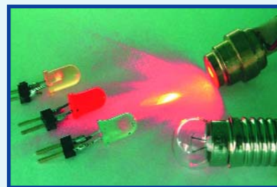
Figure 2. LEDs detecting instead of generating light.
