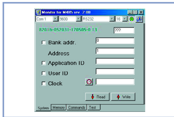
Figure 6. The monitor program M485 is used to connect to the Delphi Stamp.
