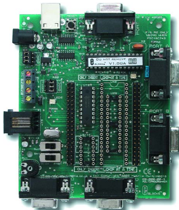
Figure 1. The USB Multiprogrammer is at the heart of the system.
