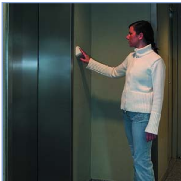
A fingerprint sensor next to a door can be used to control access.
