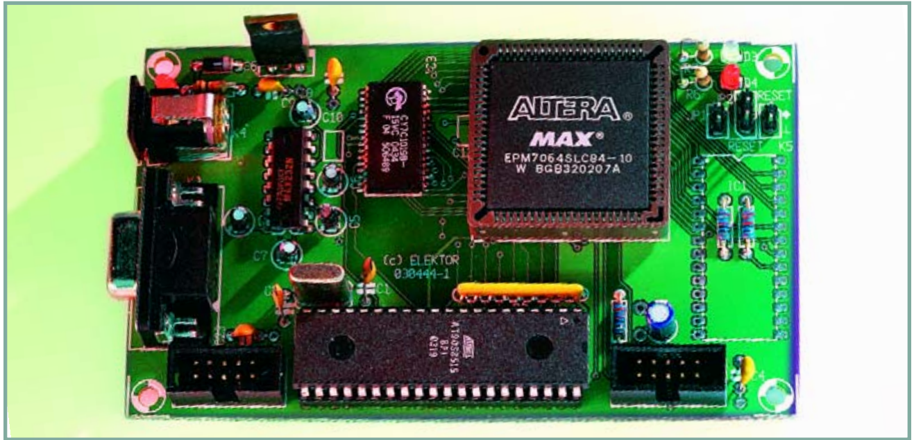
Figure 8. Fully assembled emulator prototype. It differs slightly from the final PCB supplied by us. Note the especially small dimensions of some of the capacitors (including the 1- \mu F types).
