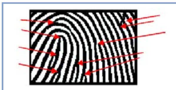
Figure 10. The so-called 'minutiae' are particular points on the finger ridges such as bifurcations and crossovers. To compare prints it is sufficient to record the position and orientation of each. (Source: Fidelica)
