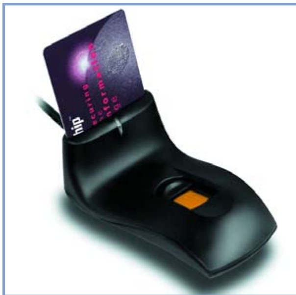
A combination of fingerprint sensor and smart card can give even greater security. It is very hard to analyse what is going on in the processor. (Source: Upek)
