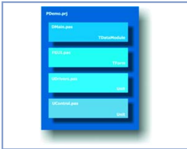
Figure 3. PDemo.prj is the container with all files that are in the Delphi simulation project.
