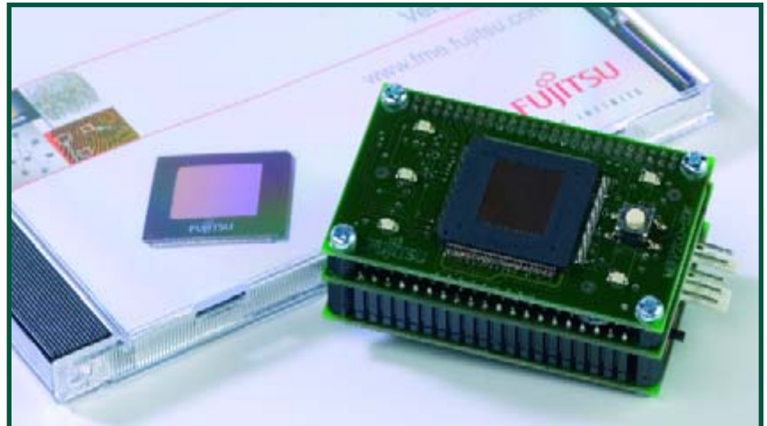
Figure 3. Fingerprint module from Fujitsu with powerful 32-bit microcontroller for autonomous applications.
