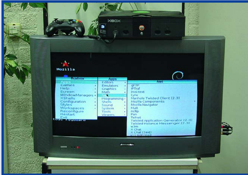
Figure 3. The modded Xbox in action (running the Live version of Xebian).
