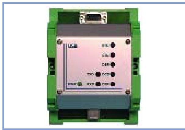
Figure 3. The Kolter adaptor, designed for mounting on a DIN rail, uses the FTDI FT8U232AM.
