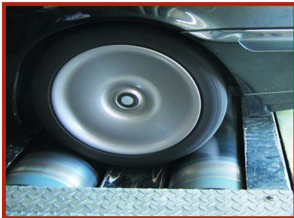
On the rolling road we increase the speed until the rev limiter kicks in.
