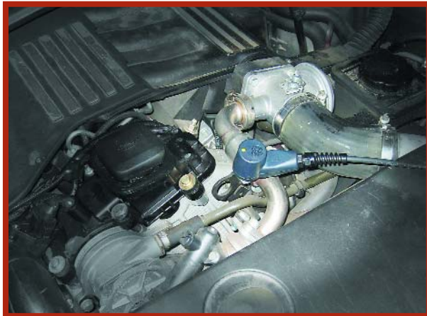
A special sensor extracts the rpms of the engine from the vibrations.
