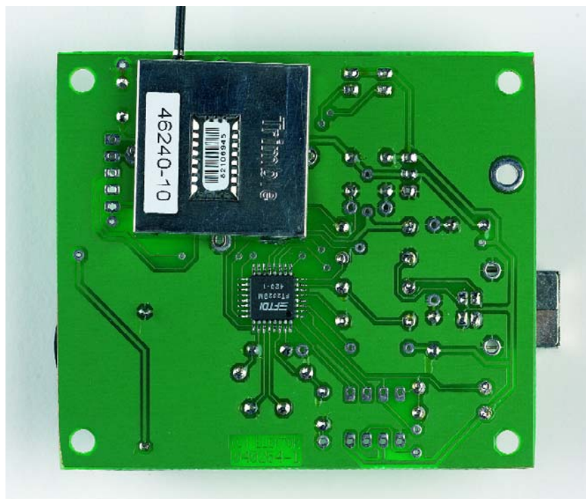
Figure 4. The IC and the GPS module are fitted to the underside of the printed circuit board.
