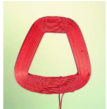
Figure 3. The author's original pick-up coil.
