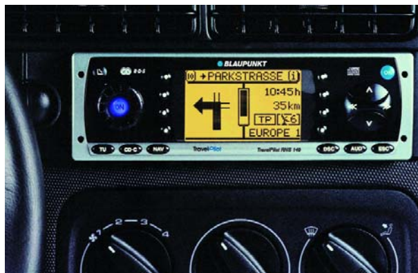
Figure 1. The TravelPilot RNS 149 from Blaupunkt crams a car radio, CD player and navigation system into a standard DIN vehicle radio-housing format. (photo: Blaupunkt)
