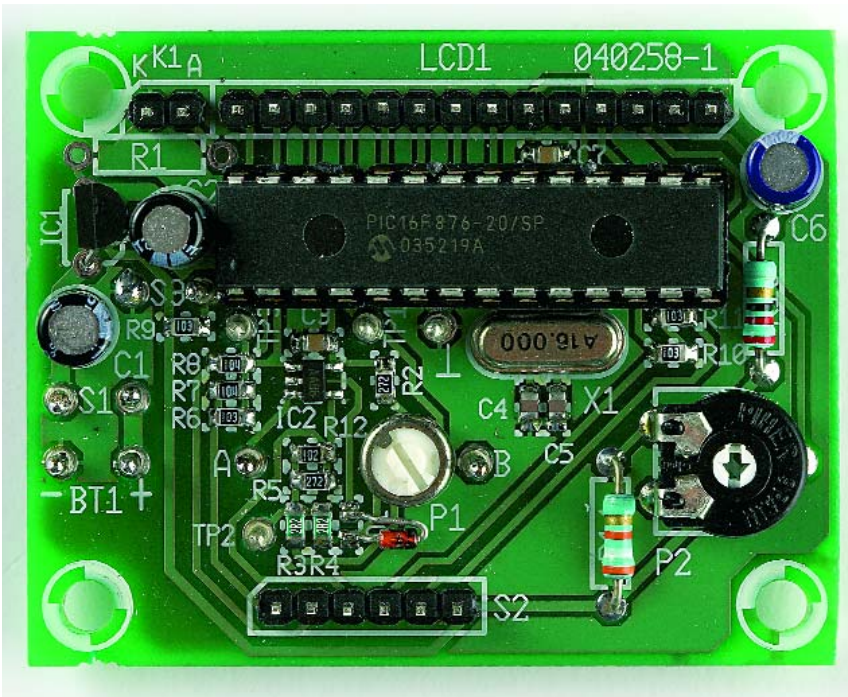
Figure 3. The finished board, ready for fitting inside the plastic case. We did not use a reset switch; instead, a 10-microfarad electrolytic cap was connected across the pins for S3. Also note the use of a leaded BAT85 instead of the SMD diode.
