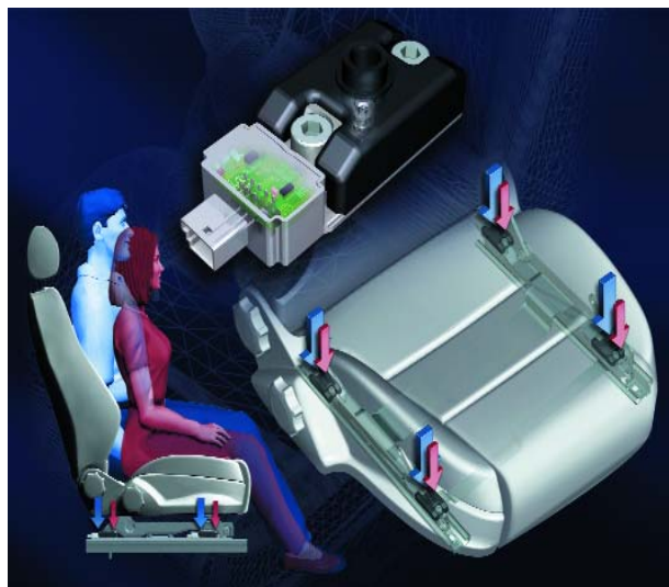
Figure 7. Electronic seat occupancy detection using force sensors at the attachment points. (Source: Siemens-VDO)
