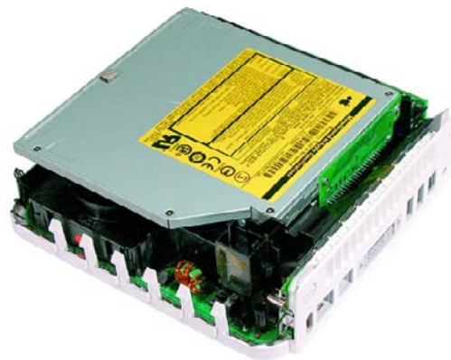
Figure 3. Inside the Mac Mini. At the top is the ultra-slim optical drive, behind which hides the 2.5" hard disk. Below, to the left, part of the centrifugal black CPU fan can be seen. Above and to the right is the main memory: a standard PC2700 DDR DIMM with 184 pins.
