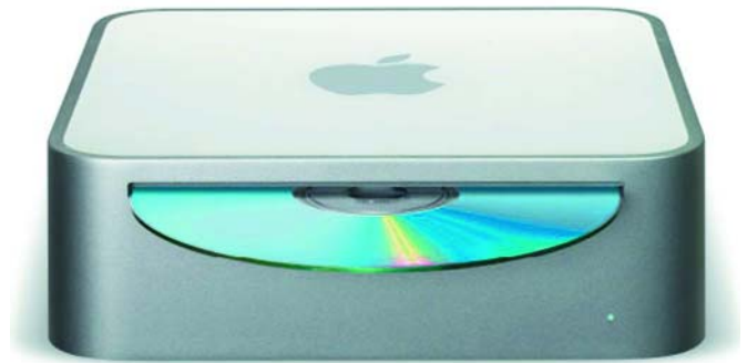
Figure 1. The Mac Mini seen from the front. A typical Apple design: nothing to see except an indicator light, a slot for optical media, and the Apple logo.
