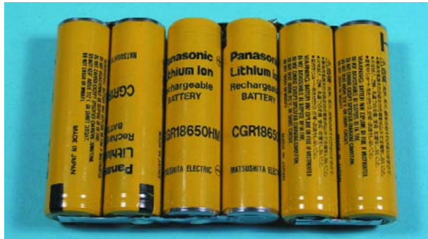
Figure 5. Li-ion battery for laptops in 3S2P configuration (10.8 V terminal voltage)
