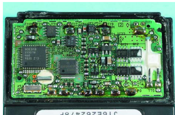
Figure 2. The integrated monitoring circuits in industrial lithium batteries are always microprocessor-controlled.
