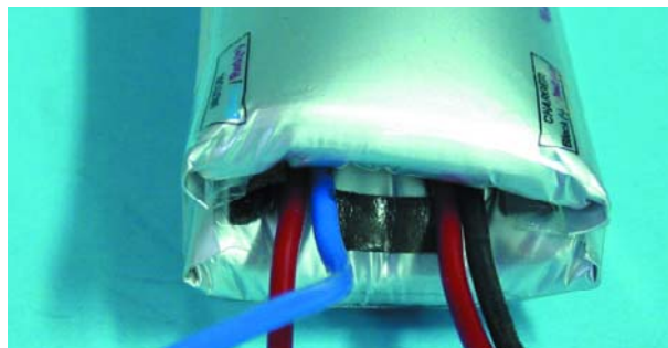
Figure 1. When a Li-polymer battery has ruptured, it is useless. In extreme cases, the battery can explode.
