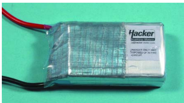
Figure 8. A wide piece of tape serves as a strain relief for the connection wires.
