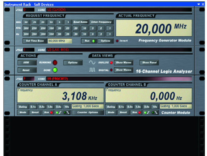
Figure 3. With these virtual instruments you can make measurements inside the FPGA.
