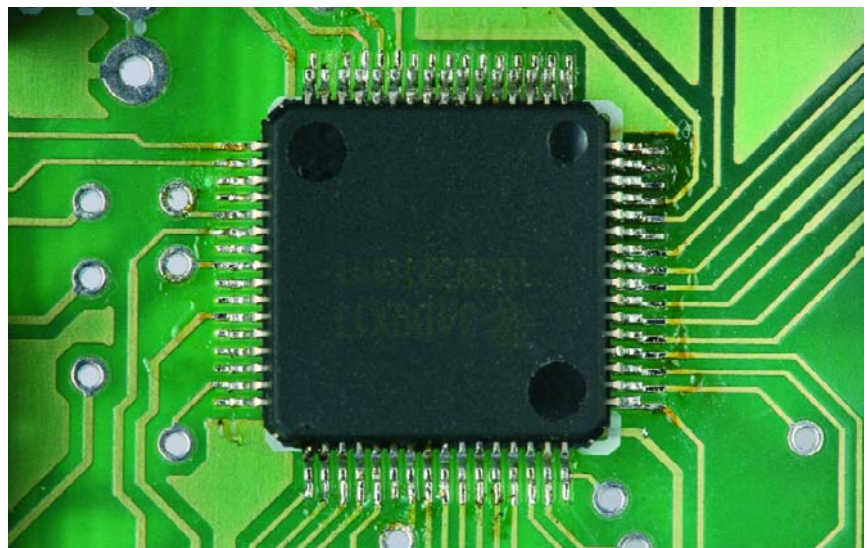
Figure 6. Tiny and tricky to solder: the USB microcontroller comes in a 64-lead SFP package.
