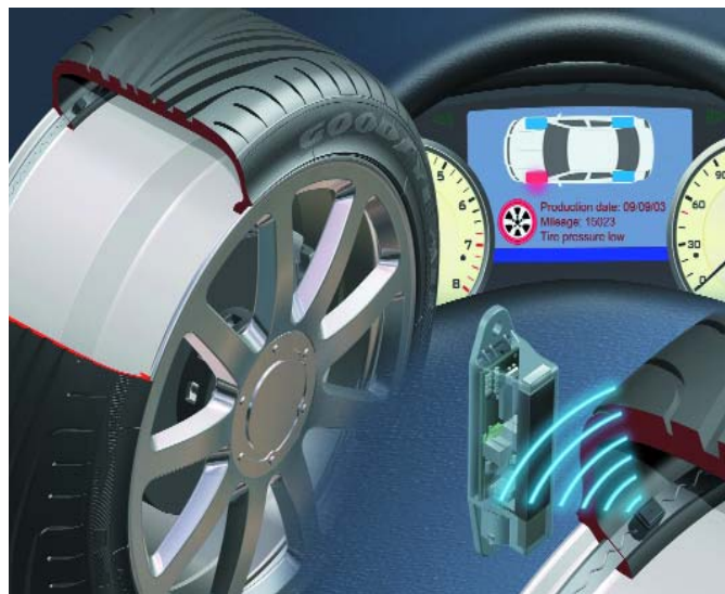
Figure 3. No more batteries in the future: passive-sensor interrogation using RFID techniques (Siemens/Goodyear).
