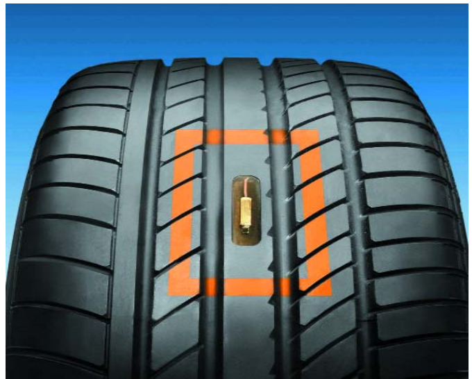
Figure 5. The 'Darmstadt tyre sensor' measures road contact by interpreting tyre profile deformation.
