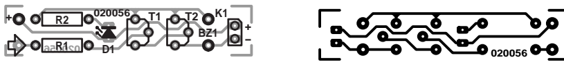
Figure 1. The narrow board and the two miniature batteries together fit into a metal tube to make a probe-like enclosure for the tester.
