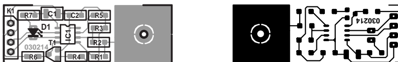
Figure 3. Copper track layout and component mounting plan of the tiny PCB designed for the circuit.
