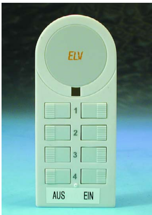
Figure 1. The handheld transmitter (ELV part code FS 10 S8-2) before modification.
