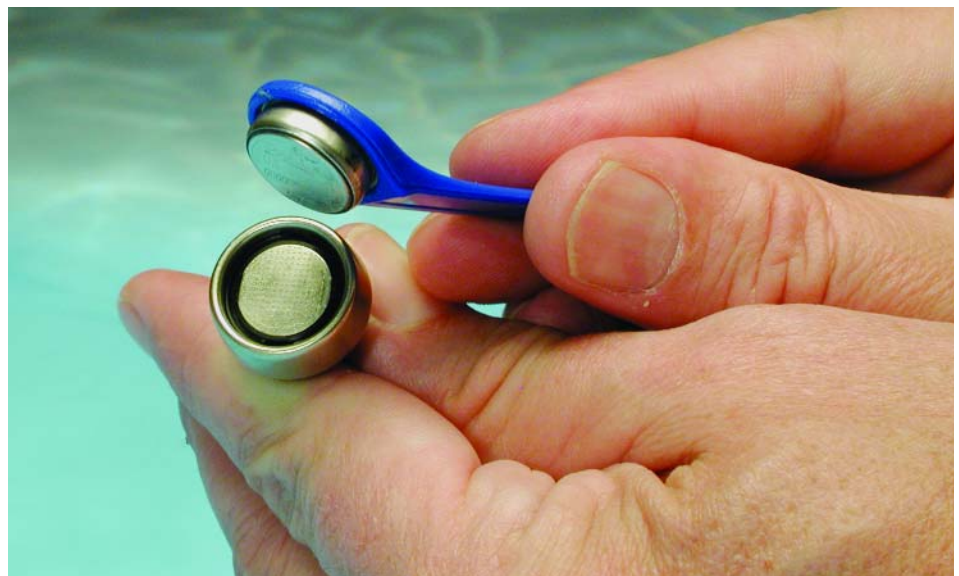
Figure 1. A DS9092 iButton with associated read probe.
