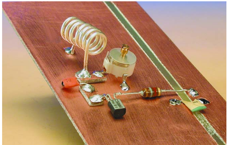
Figure 4. With a few homemade islands, a complete circuit can be built quite quickly using the Manhattan method, which may be described as an RF-optimised variant of Ugly Construction.
