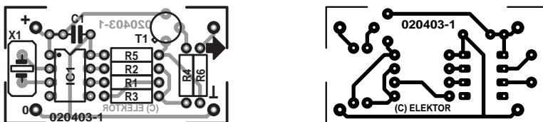
Figure 3. Layout and component overlay for the printed circuit board for the mini test chart generator.
