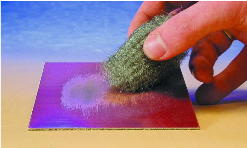
Figure 1. The printed circuit board material must always be scrubbed to obtain a clean surface.
