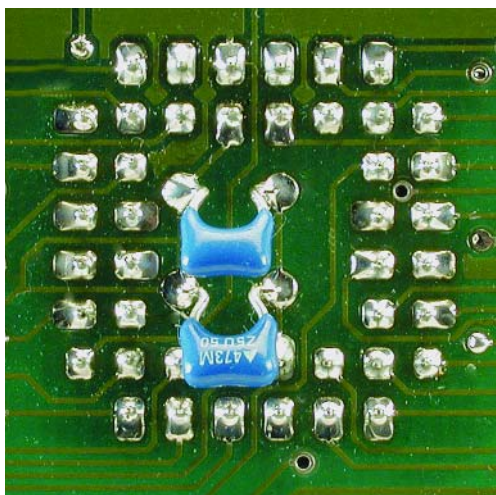
Figure 3. Close-up of the placement of C1 and C2 at the solder side of the board.
