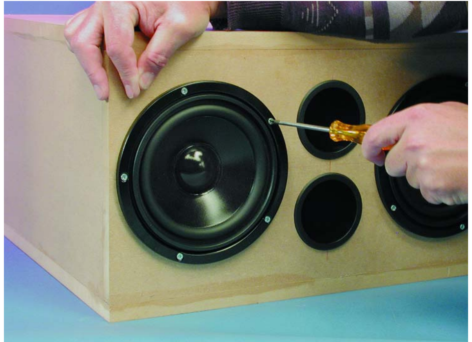
Figure 5. The woofers have to be screwed down tight to avoid unwanted resonance.
