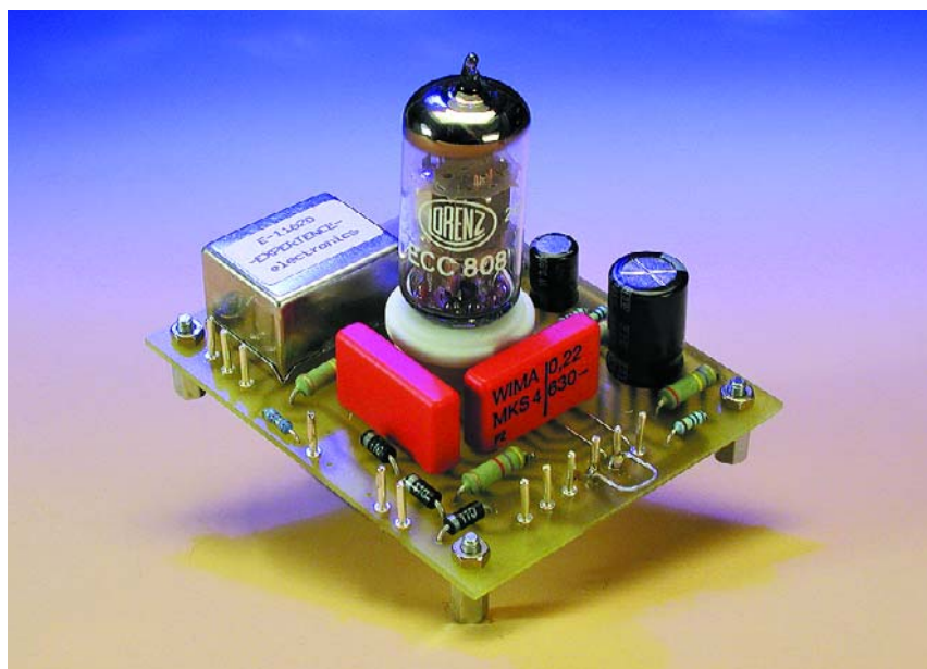
Figure 8. Circuit board layout for ECC808 (board available from Experience Electronics).
