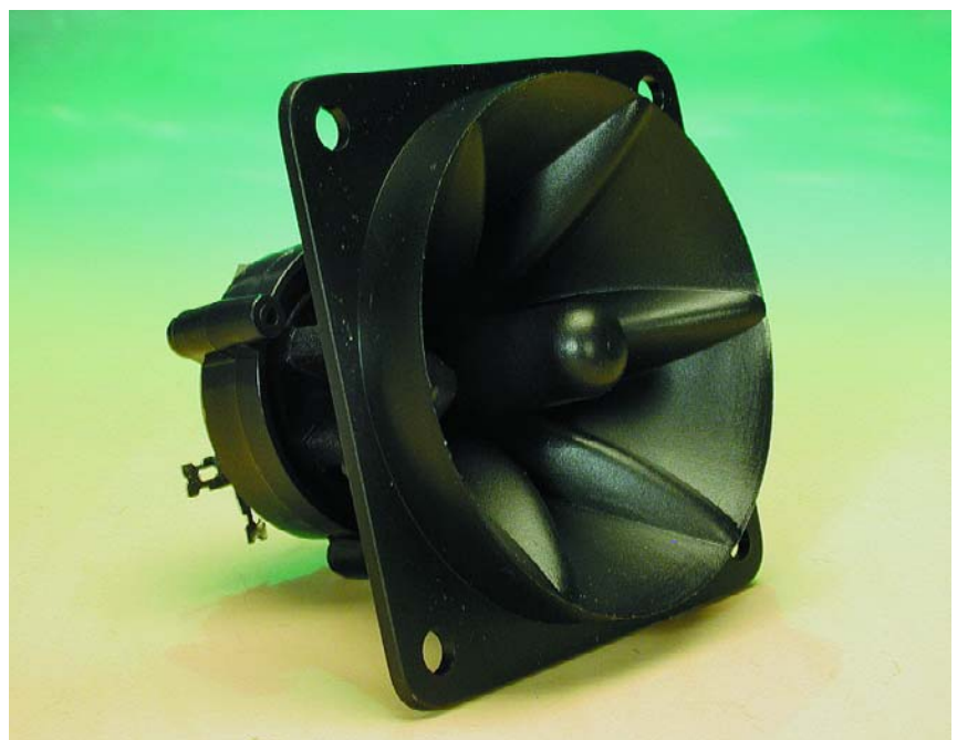
Figure 4. The piezo tweeter used for the prototype is a type PH8 from Visaton, it has a frequency range from 3 kHz to 40 kHz and is capable of producing very high sound pressure levels.
