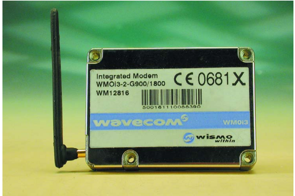
Figure 1. Heart of the project: the ready-programmed GSM modem supplied by Unitronic.
